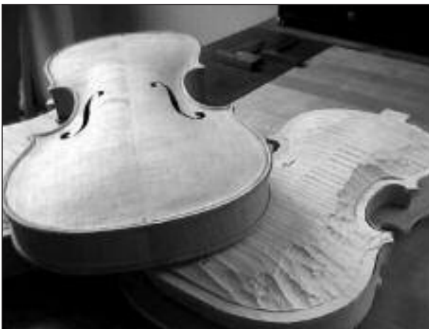
A violin body in the early stages of carving (right) compares starkly to one that is near completion. Photo by Marolyn Taylor.
